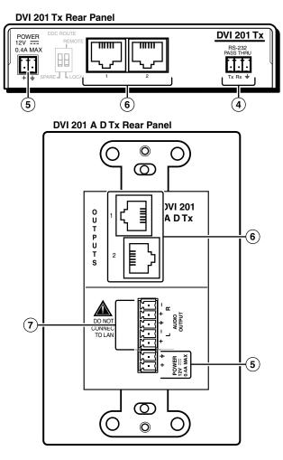
Figure 2-13 — DVI 201 Tx rear panel connectors
